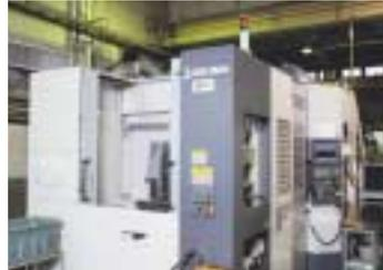
Precision machining of parts on a horizontal MC
