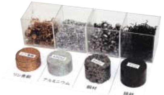
Thanks to a chip compressor that was developed in-house (sold externally), there is not a single chip storage bucket taking up space in our Yamagata plant
