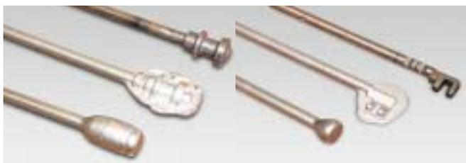
▲"Electric upsetting," which enables plastic forming of bar material in any location, contributes greatly to making products more lightweight and eliminating processes (photo shows fork shafts for manual transmission. Finished products are at top.)
