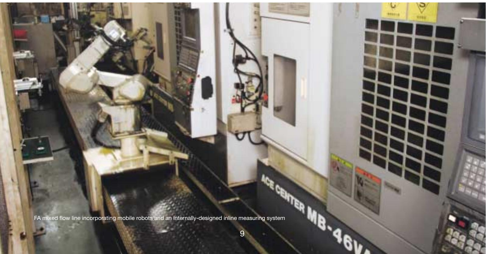
FA mixed flow line incorporating mobile robots and an internally-designed inline measuring system
