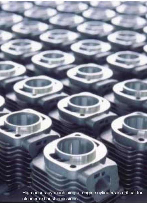
High accuracy machining of engine cylinders is critical for cleaner exhaust emissions
