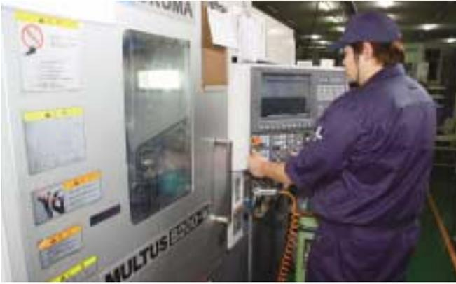
Process-intensive machining on a single MULTUS B200-W of bar material that was previously done in six processes on multiple machines
