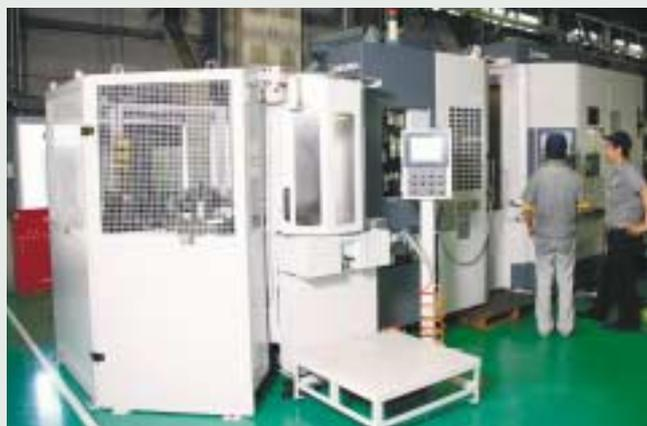
At Tec Nagasawa, MA-400HA was the first horizontal machining center. Equipped with 6 pallets, the tool magazine can store 160 tools.
