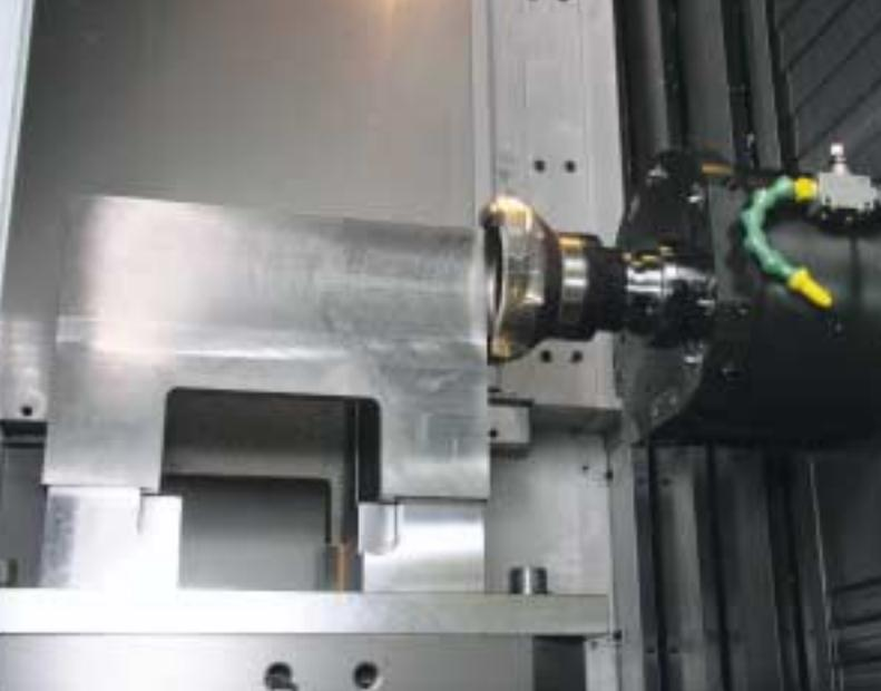
When extracting the optimum conditions with the "Machining Navi" while face milling vacuum chamber parts, the tool life becomes approximately twice as long.
