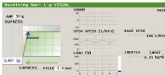
With a visualization of the machining sounds and spindle load, you can increase spindle rotation even more and improve productivity.
