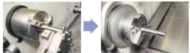
When using a steadyrest (left), it can leave roller marks on the workpiece or cause swarf buildup, but with the Machining Navi (right), you don't need to use a steadyrest.
