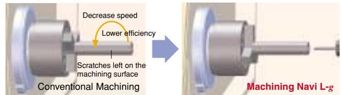
**Machining efficiency is 1.5 times higher without the steadyrest.**
