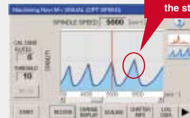
**If you can find the right conditions on a long tool, it is possible to machine many points on the same tool.**
