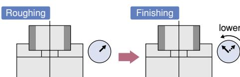
for finishing, there is no bother using a pusher as with horizontal lathes. Chucking warp is also prevented.
