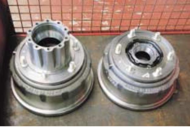
Hub and drum assemblies are important safety parts that demand high accuracy machining
