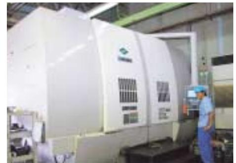
2SP-V80 turning underbody parts of  $\phi 800$  mm.
