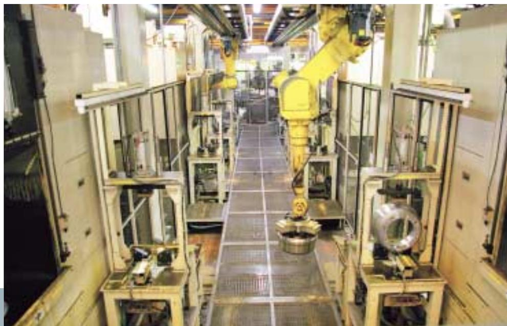
Brake drum machining line with 6 vertical lathes and robots
