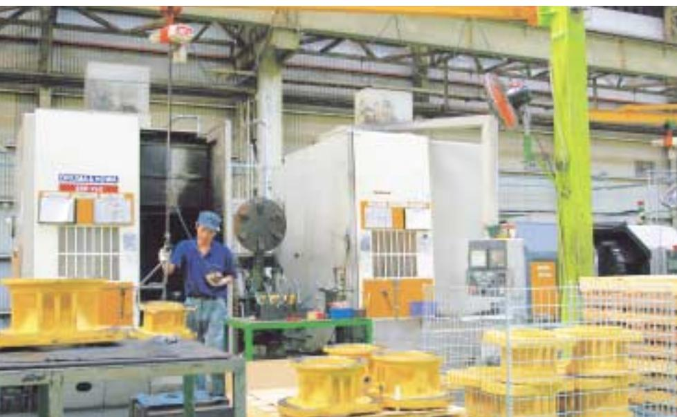
Lead time shortened and work in process storage areas greatly reduced with a line consisting of a 2-spindle vertical lathe and a machining center
