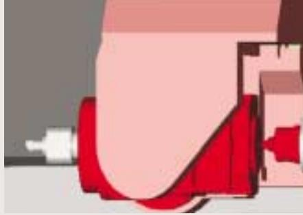
If attention is focused only on the tool tip, a collision with the cover or tailstock may occur
