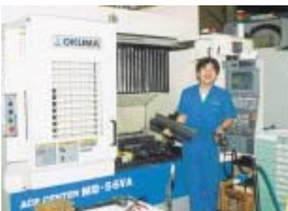
next brought in an MB-56V to do something about the thermal deformation that was giving us such a hard time. Up to that point we had had thermal deformation of 20-30 microns, which we had to deal with through compensations several times each day. Thanks to the MB-V, we are now okay to go with a single measurement in the morning. This really surprised our people on the shop floor. Productivity has improved dramatically.
