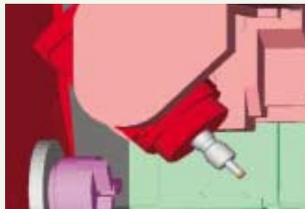
Machine stops before interference. Trial cutting is greatly reduced.
