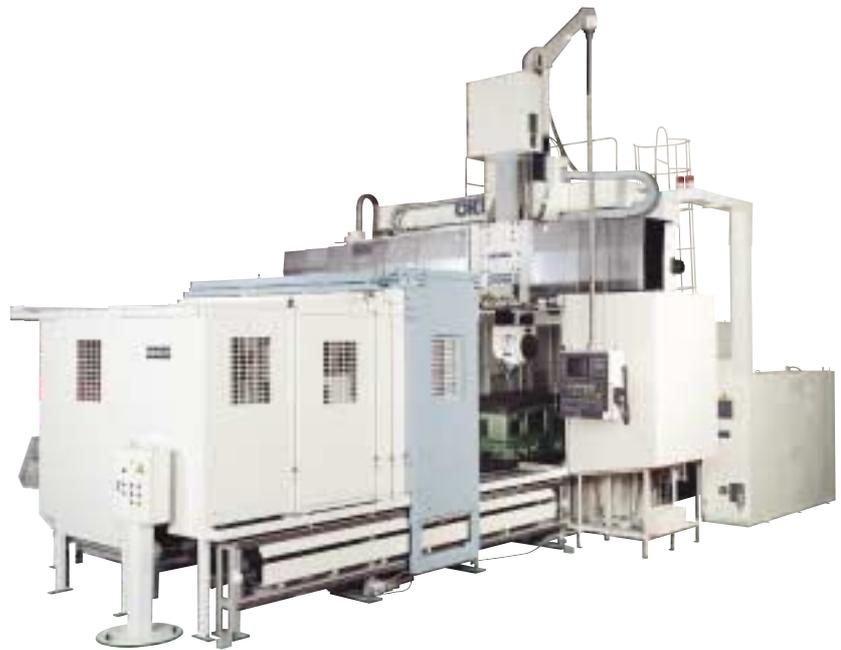
5-sided machining expert MCR-BII (high-speed, high-accuracy specs) with stainless-steel tank and full-enclosure shielding in support of ecological concerns.
