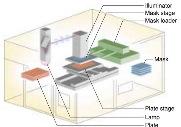
A large-plate exposure system. An ultra-precise machine with a loader to assemble the illuminator, mask, and plate at a stage.
