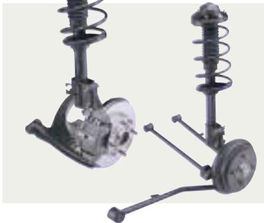
The steering knuckle – plays an important role in the suspension of a car (2 locations) to insure safe motoring.
