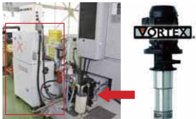
The "Vortex" (2011 Good Design Award recipient) replaces a large coolant supply pump and tank (left) with an integral-type pump
