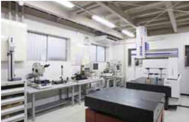
Stringent check with precision measuring instruments for dimensional accuracy, roundness, surface roughness, and contour shape in the inspection room.
