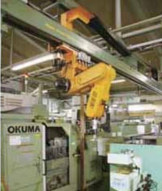
Many manufacturing processes are automated. Loaders, robots, and control systems are made in-house. The cylindrical grinder is a production type GA-25T.
