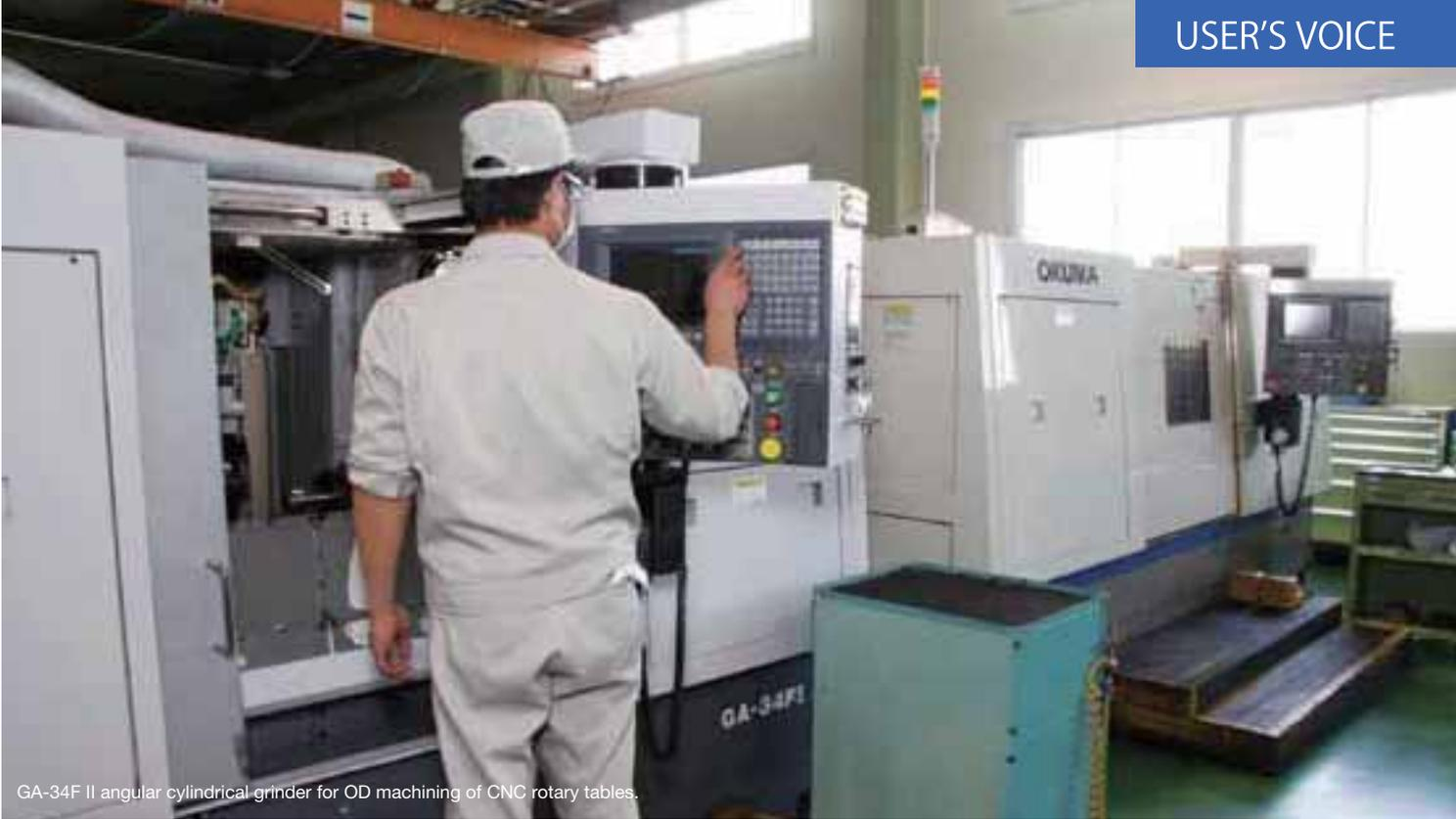
GA-34F II angular cylindrical grinder for OD machining of CNC rotary tables.
