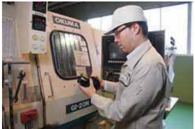
GI-20N internal grinder performs ID finishing operations mainly on collet chucks
