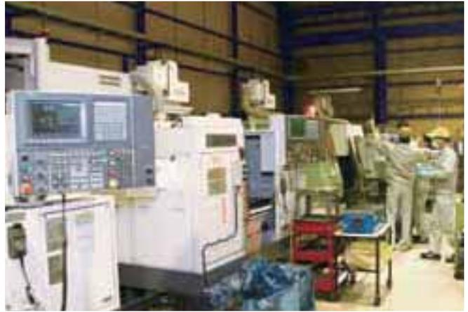
CNC cylindrical and internal grinders support super-precision machining that corresponds to a wide variety of bearing parts.
