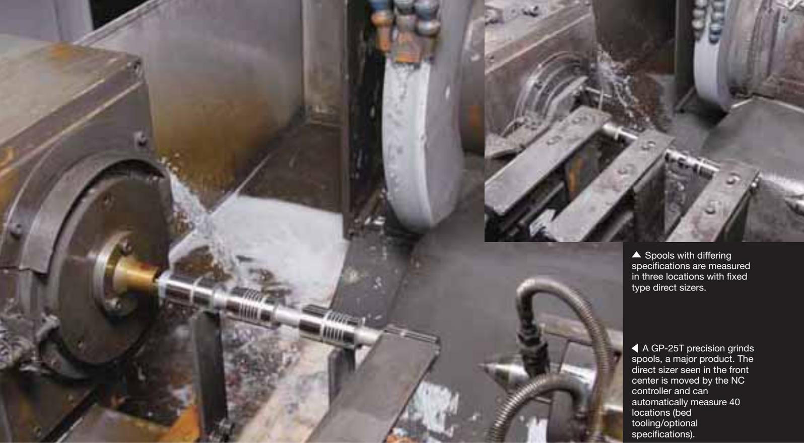
▲ Spools with differing specifications are measured in three locations with fixed type direct sizers.
