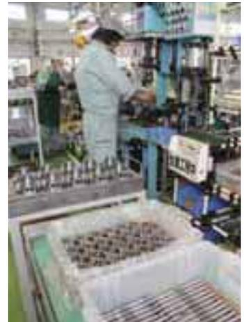
Precision machined shafts are sent to the pump assembly line.
