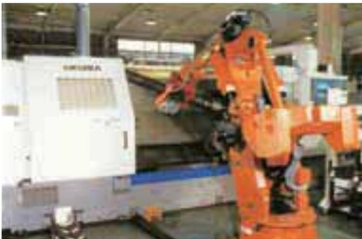
Hydraulic cylinder tube machining line (Headquarters)
