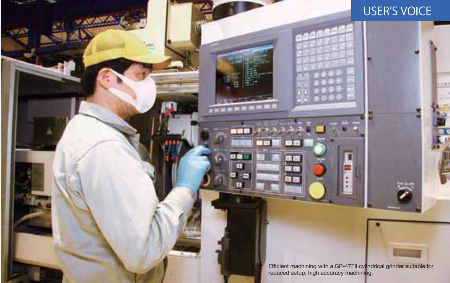
Efficient machining with a GP-47FII cylindrical grinder suitable for reduced setup, high accuracy machining.
