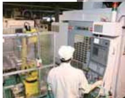
Higher productivity with use of "Machining Navi" intelligent technology on machining centers
