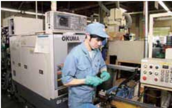
The GI-2N-SP ultra-precision, compact, internal grinder handles mass production and grinds pinion gears at a rate of about one per 10 sec. Most of the external measuring equipment, carriers, and other parts of the automation system were designed in-house by Fujieda Kenma Kogyosho.
