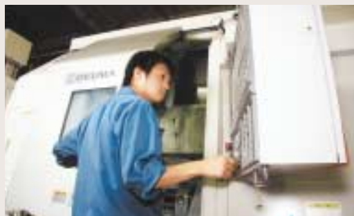
One of our young experts, Mr. Kageyama, frequently makes adjustments to the spindle speed by matching it carefully with the noise and oscillations.
