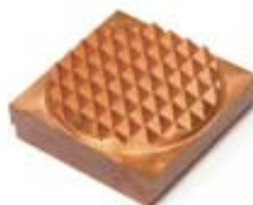
Left: Sample of a machined square pyramid without burrs, that is 6 mm tall, made from a machining center. Right: Polyhedron machining created from 2011 small flat surfaces using cutting processes with an NC lathe and a 5-axis machining center.
