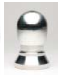
Left: Sample of a machined square pyramid without burrs, that is 6 mm tall, made from a machining center. Right: Polyhedron machining created from 2011 small flat surfaces using cutting processes with an NC lathe and a 5-axis machining center.
